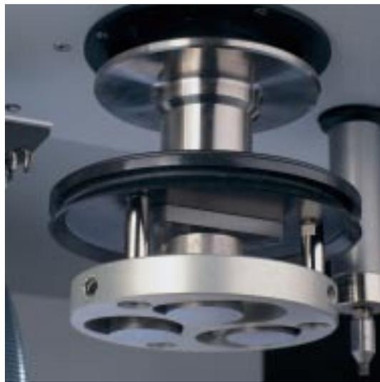
*Prepamatic-2 can handle both single specimens and specimens clamped in holders*
